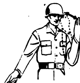
Turn to left (port). Position right arm down and point to left wheel; move left arm repeatedly upward and backward. Indicate rate of turn by rapidity of arm motions (STANAG 3117).
